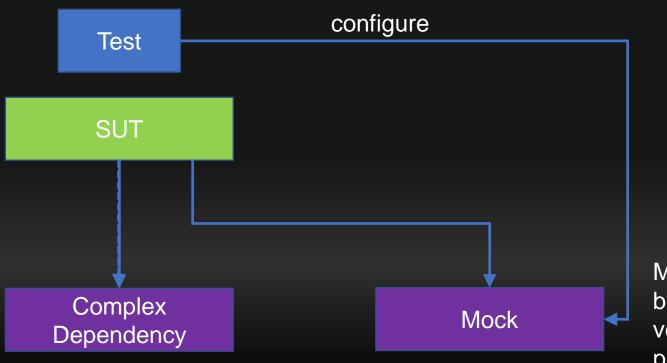
Mock provides same interface but can be configured to verify inputs and produce preprogrammed outputs
